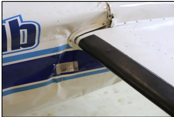
Photos No. 4 & 5: Significant structural damage to either side of the rear fuselage
