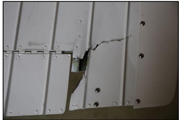
Photo No. 3: Tear to trailing edge skin
