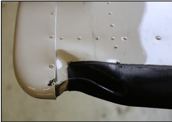
Photo No. 2: Leading edge indentation
